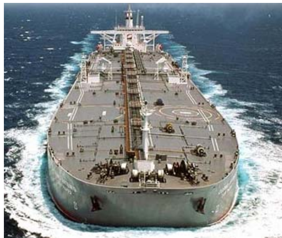
Stopping a supertanker: it takes 14 minutes and three kilometres once you decide to alter course or speed, before the manoeuvre is complete.
